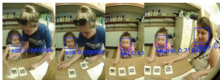
Fig. 15: This figure shows the emotion detector CNN working on previously recorded ABA therapy sessions by PABI.
